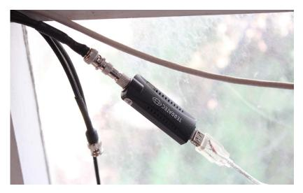
One can purchase purpose built hardware or a TV dongle as pictured at right for (in my case) \$20 off of eBay, even less from China. I run the device on a Debian box which has GNURadio compiled and installed. The images below are from a Win7 box running SDR# which is free software that can either drive the device directly or access across a network which is what I do. Makes for convenient antenna / cable / machine placement.
